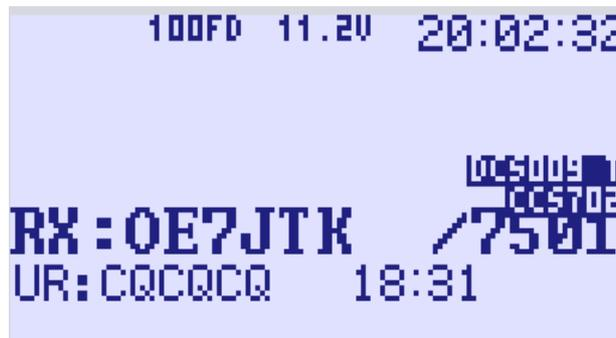
Figure 18: Display page D-STAR with connection to DCS009T and CCS-Server CCS702
